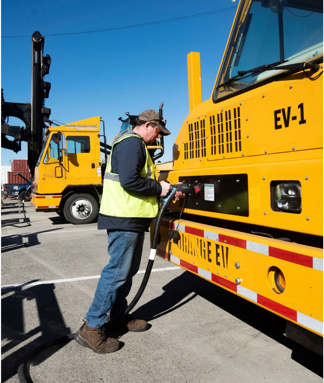
Electric yard truck at the South Intermodal Yard
